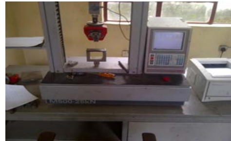
Fig 2 Testometric machine used for the test
